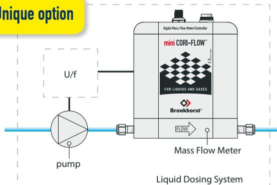
**mini CORI-FLOW™** incorporates PID control as standard
