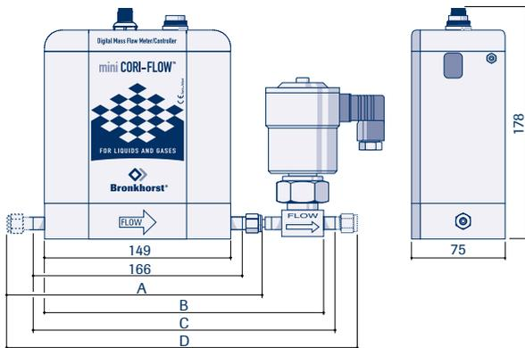
The valve in this drawing is the CSI. Other valves have different shapes.
