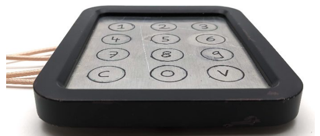
b) Top side of the touchpad with keys identified by marker drawings.
