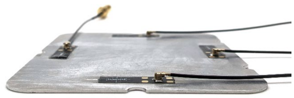
a) Bottom side of the aluminum plate with the Dragonfly sensors.
