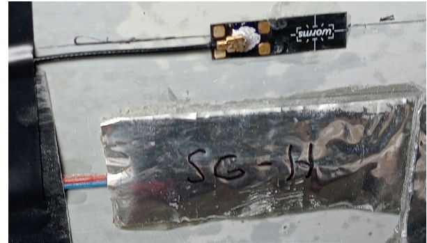
Figure 3: Dragonfly sensor before protective layer installation
