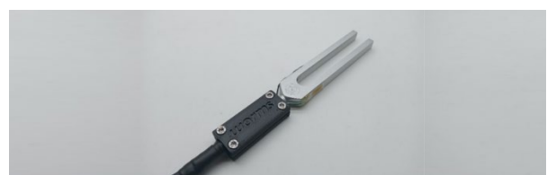
Figure 1: Tuning Fork equipped with a strain gauge and a Dragonfly®
