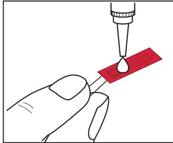
Ascertain the back and front of the strain gage. Apply a drop of adhesive (CC-33A) to the back of the strain gage.
