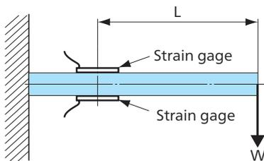
Bending Stress Measurement with Half-bridge System
