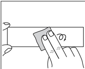
Using a sand cloth (#320), polish the strain-gage bonding site over a wider area than the strain gage size. Wipe off paint, rust and plating, if any, with a grinder or sandblast before polishing.
