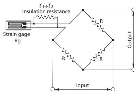
Bridge Circuit Designed with Insulation Resistance
