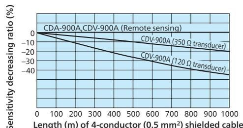
Note that the CDV-900A has a built-in remote-sensing circuit, and thus use of a 6-conductor (0.5 mm²) shielded cable prevents the sensitivity from decreasing up to approximately 2 km. For the remote-sensing method, see page 9-14.
