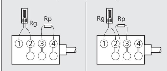
Precaution: Avoid inserting  $R_p$  to the side where the strain gage is connected. Such connection adversely affects the sensitivity.
