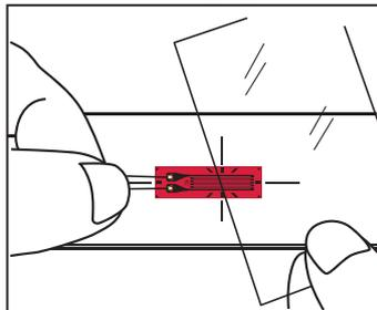
After applying a drop of the adhesive, put the strain gage on the measuring site while lining up the center marks with the marking-off lines. Cover the strain gage with the accessory polyethylene sheet.
