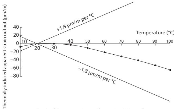
Typical Temperature Characteristics of Self-temperature-compensation Foil Gage
