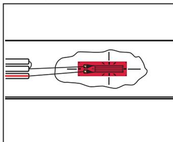
After pressing the strain gage with a thumb for one minute or so, remove the polyethylene sheet and make sure the strain gage is securely bonded. The above steps complete the bonding work. However, good measurement results are available after 60 minutes of complete curing of the adhesive.
