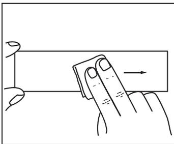
Using an industrial tissue paper dipped in acetone, clean the gage bonding site. Strongly wipe the surface in a single direction to collect dust and then remove by wiping in the same direction. Reciprocal wiping causes dust to move back and forth and does not ensure cleaning.
