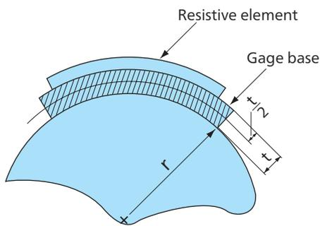
Strain Gage Bonded on the Curved Surface
