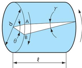
When the axis is twisted, point A moves to point B, thereby initiating torsional angle  $\theta$ .
