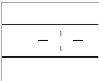
Mark the measuring site in the strain direction. Use a 4H pencil or a marking-off pin. When using a marking-off pin, take care not to deeply scratch the gage bonding surface.
