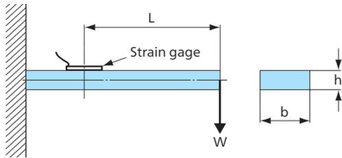
Bending Stress Measurement with Quarter-bridge System
