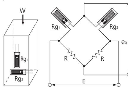
Tensile/Compressive Stress Measurement with Half-bridge System
