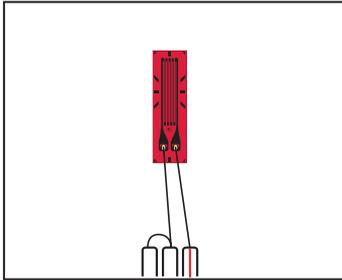
Select the strain gage model and gage length which meet the requirements of the measuring object and purpose. For the linear expansion coefficient of the gage applicable to the measuring object, refer to Linear Expansion Coefficients of Materials (page 9-1).
