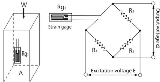
Tensile/Compressive Stress Measurement with Quarter-bridge System
